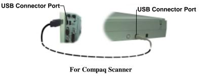
2. Plug the other end of this cable into the port located on the back panel of the scanner.
